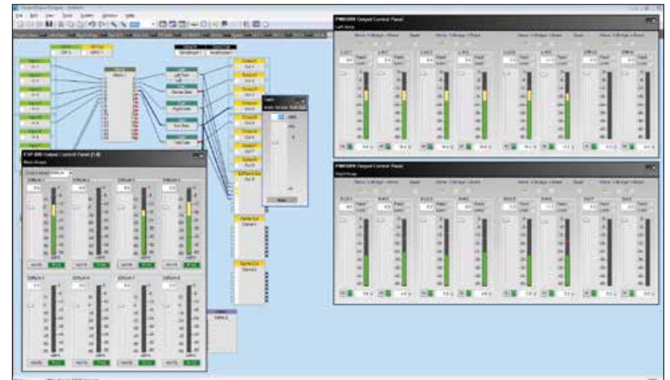
Real-time network monitoring of multiple amplifiers
